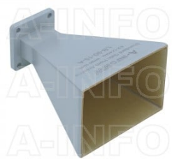
LB-90-15-A Standard Gain Horn Antenna 8.2-12.4GHz 15dB Gain Rectangular Waveguide Interface
